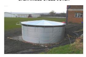
Manufactured using Z35 galvanised 1.6mm sheets this steel sectional roof complete with access hatch and ball valve cover offers a secure safe solution as well as being aesthetically pleasing. The galvanised steel cover is designed and manufactured to complete with BS5950, BS5502
