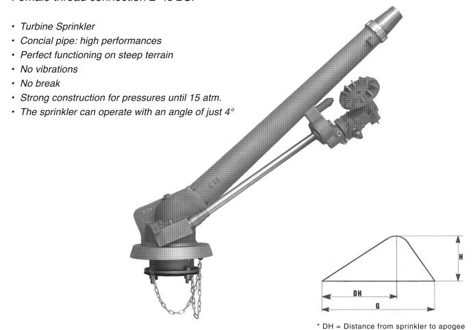
Lenght of jet G Distance DH\* Nozzle Pressure Discharge Apogee H Ømm atm. I/min 31 - 35 - 37 26 4,0 - 5,0 - 6,0 860 - 957 - 1060 47 - 51 - 53 17 - 19 - 21 28 4,0 - 5,0 - 6,0 997 - 1110 - 1225 49 - 54 - 57 18 - 22 - 25 32 - 38 - 40 30 5,0 - 6,0 - 7,0 1237 - 1394 - 1520 56 - 57 - 58 21 - 24 - 26 39 - 40 - 41 40 - 42 - 43 32 5,0 - 6,0 - 7,0 1475 - 1587 - 1735 61 - 63 - 66 22 - 25 - 27 34 5,0 - 6,0 - 7,0 1645 - 1792 - 1935 62 - 64 - 67 23 - 25,5 - 27,5 41 - 43 - 44 25 - 29,5 - 34
