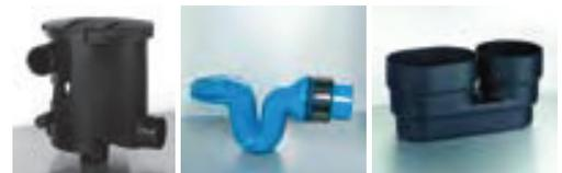
**Kit C;** Will service an 800m2 roof area and has exactly the same filter mechanism as Kit B - again this filter should be cleaned twice a year. 100mm connections, 0.65mm stainless steel mesh. This kit would generally be used on tanks between 5,500 - 20,000ltrs.
