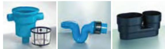
**Kit B;** Will service a 450m2 roof area and is better suited for WC flush and a better quality of water filtered, this filter can also be used for general garden use, vehicle washdown, dairy and much more... This filter should be cleaned twice a year depending on contamination. 100mm connections, 0.65mm stainless steel mesh. This kit would generally be used on tanks between 5,500 - 20,000ltrs.
